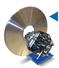
Caliper Disc Brakes offer the most flexible approach to braking because disc size and number of calipers can be combined to offer the desired torque within a given envelop parameters. Built in sensors detect brake status (on/off), wear adjust and friction pad wearout.
