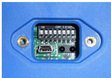
Figure 11: Dip switch block as viewed through USB/IR port
