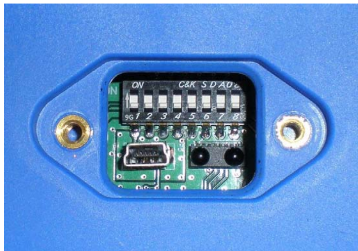
Figure 8: Dip switch block as viewed through USB/IR port
