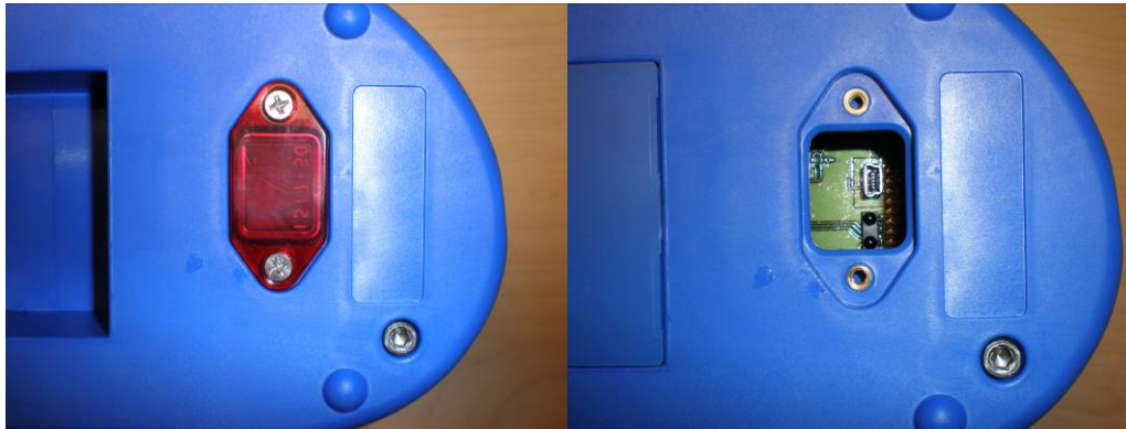
Figure 7: USB/IR Cover Location and Cover Removal
