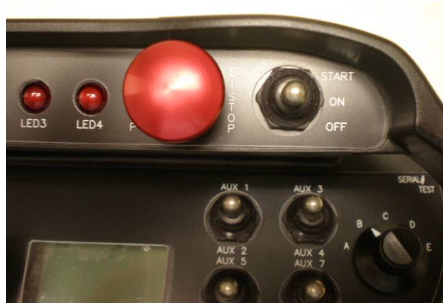
Figure 5: Machine Stop Switch and OFF-ON-START Toggle
