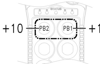
Examples:                      Press PB2 two times and then PB1 four times will give you channel 24.
