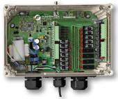
including 433MHz, 900MHz, and 2.4GHz are available, along with 1 analog and 5 digital integrated inputs.
