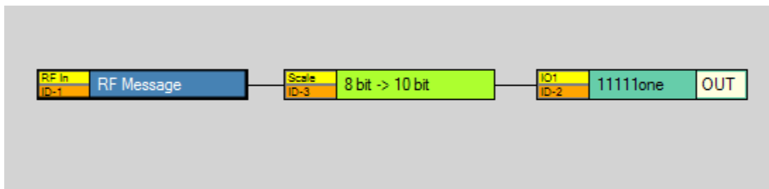
Figure 38: This example shows how to scale an 8-bit RF message to a 10-bit value to drive an output. NOTE: This is needed to achieve full scale on the output.
