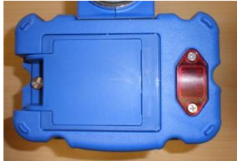
Figure 5: Installation of Battery Cover
