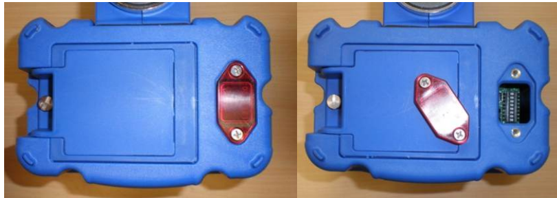
Figure 7: USB/IR Cover Location and Cover Removal
