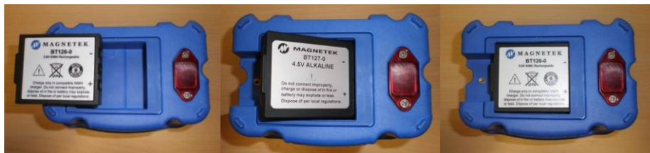
Figure 4: Installation of Battery Pack into MBT transmitter
